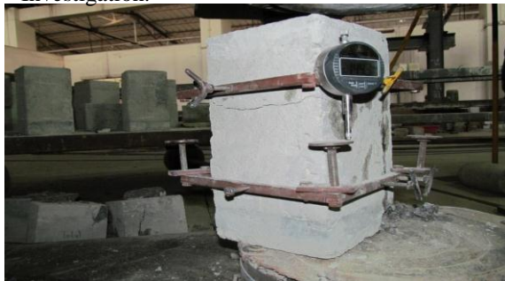
Fig. 5. Testing of prisms with 0.002 least count dial gauge
