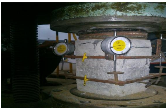
Fig. 6. Trial test of the prism with 0.01 least count dial gauge
