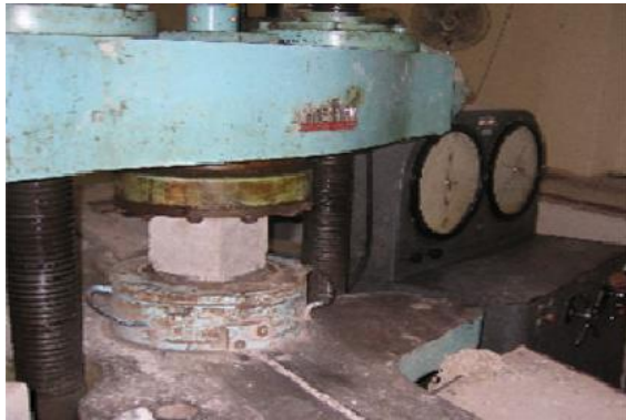
Fig. 8. Details of cube testing under TOTM
